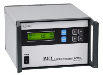
Electronic Current Burden M401 is a programmable device used as a load in the secondary circuits of Current Instrument Transformers with secondary current 5 A during their verification and calibration
