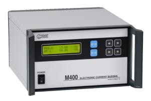
Electronic Current Burden M400 is a programmable device used as a burden in the secondary circuits of Current Instrument Transformers with secondary current 1 A during their verification and calibration
